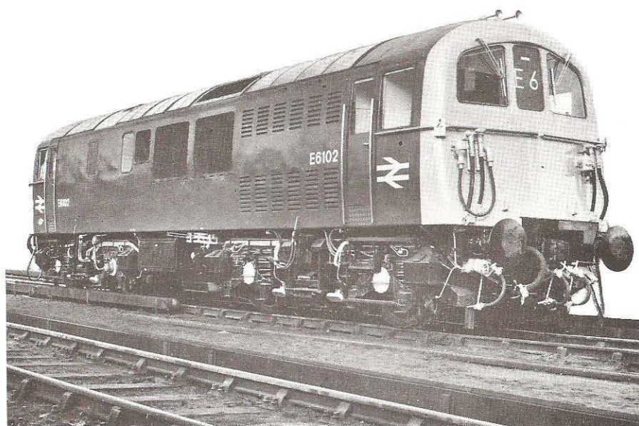
E6102 after conversion. The retractable shoe gear can be clearly seen.
